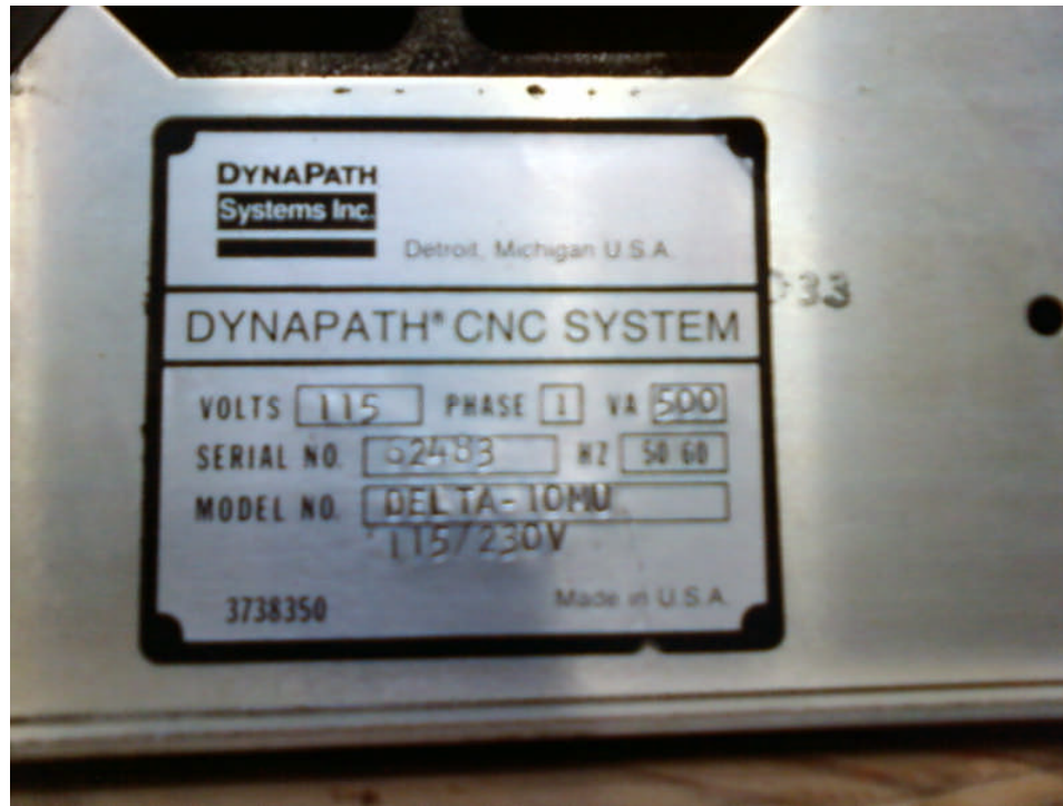
Example Control Serial Number Tag: Delta 10 Mill Control (Unbundled), S/N 62483
